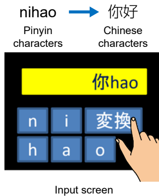
Fig. 3 Illustration of use of Chinese input function
