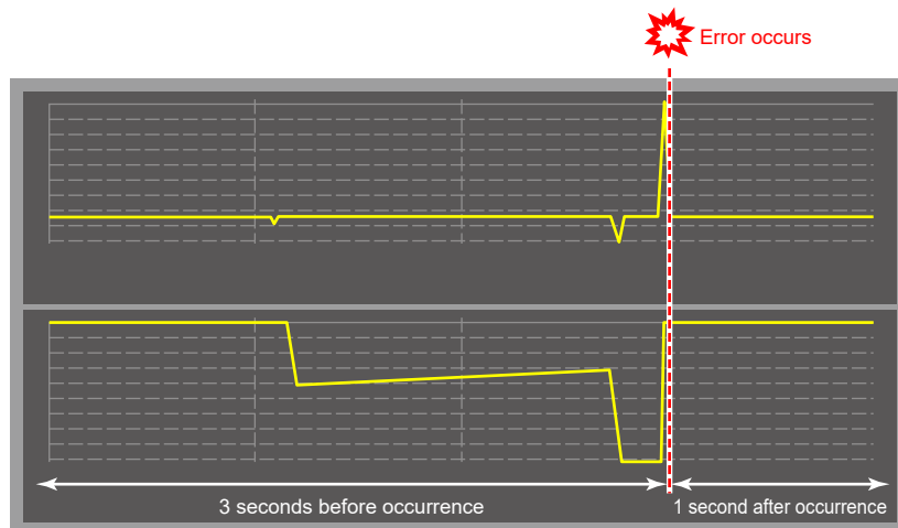
Fig. 4 Conceptual illustration of drive recorder
