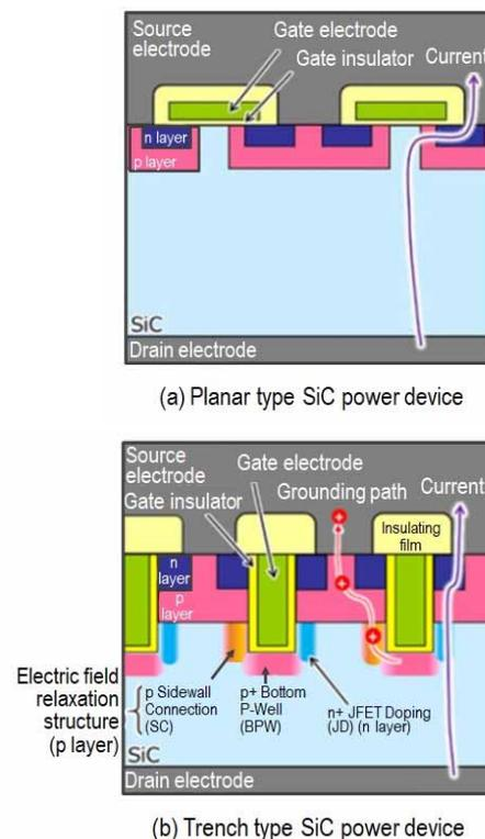
Fig. 2 Schematic diagrams of Mitsubishi Electric SiC MOSFET
