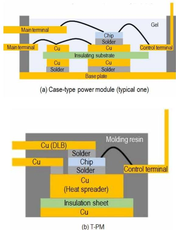
**Fig. 3 Representative example of case-type power module and package structure of T-PM**
