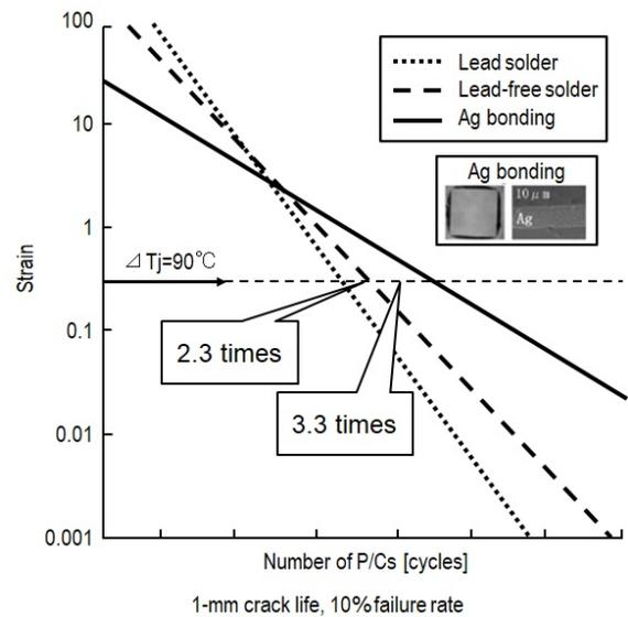
Fig. 5 Stress endurance diagram of various bonding materials
