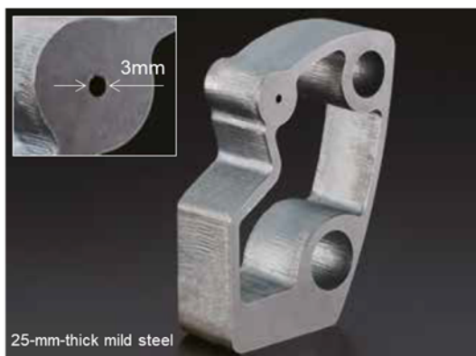
Fig. 6 Small hole processing of 25-mm-thick mild steel
