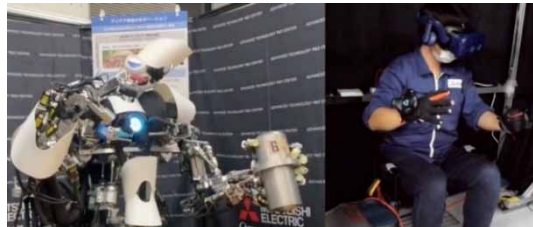
(b) High-power humanoid remote control robot that can grasp and transfer a 6-kg or heavier object with one arm
