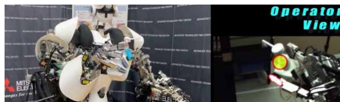
Haptic information was presented by AR even when there was a shield when the robot grasped an alcohol container.
