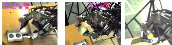
Grasping and transferring a raw egg Grasping and transferring a potato chip Grasping and transferring a card
