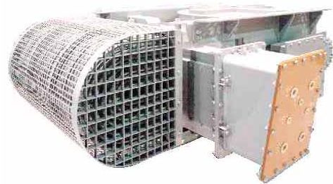
Fig. 4 Natural air cooling type transformer for type 683 train (JR-West)
