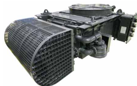
Fig. 2 Natural air cooling type transformer for type E657 train (JR-East)
