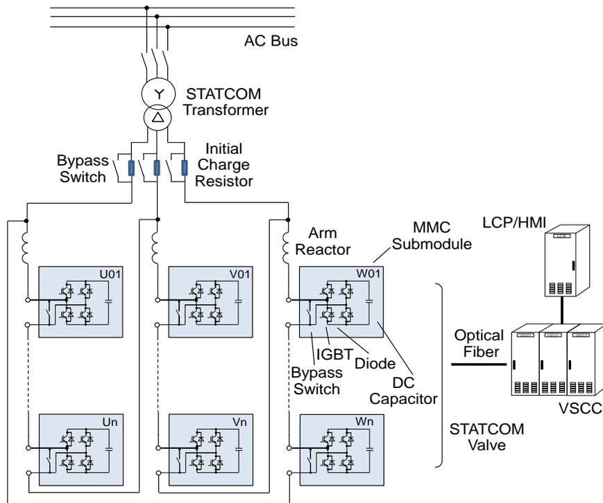
Fig. 3 Colington STATCOM system configuration
