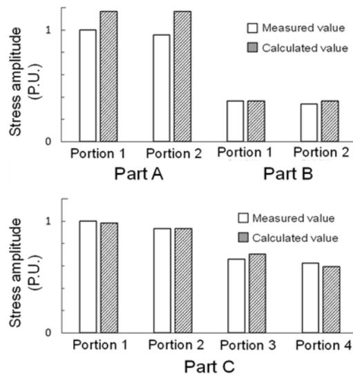
Fig. 7 Measurement results of stress on the rotor wedge and retaining ring
