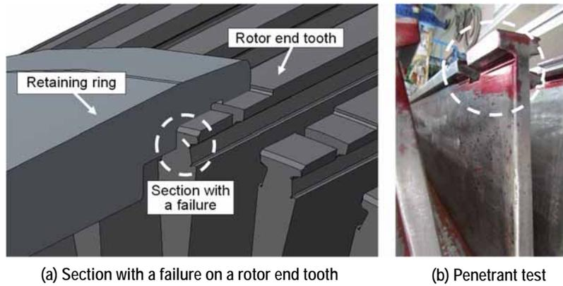
Fig. 8 Penetrant inspection of a rotor end tooth
