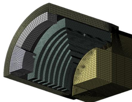
Fig. 5 Structural analysis model for a rotor end (1/4 of the circumference)
