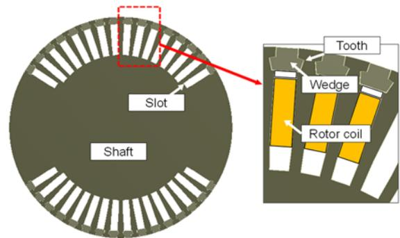
Fig. 3 Cross-section of a rotor
