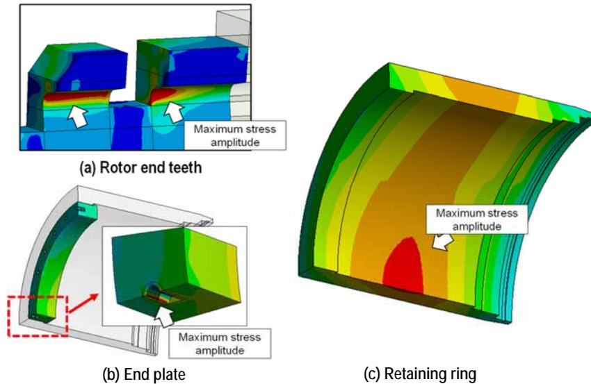
Fig. 6 Stress amplitude at the rotor end when a generator is operating and not operating
