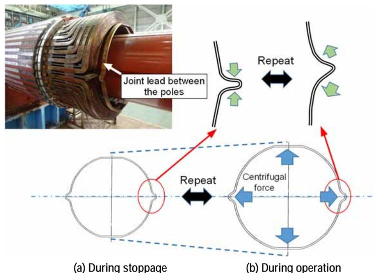
Fig. 1 Repeated stress occurring at rotor parts due to start and stop
