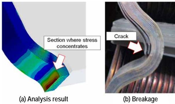
Fig. 2 Breakage of a rotor part due to low cycle fatigue
