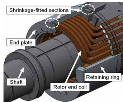
Fig. 4 Rotor end structure
