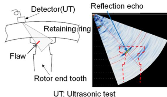
Fig. 9 Ultrasonic test of a rotor end tooth
