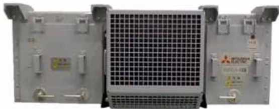
Fig. 4 VVVF traction inverter system for the 5000 series
