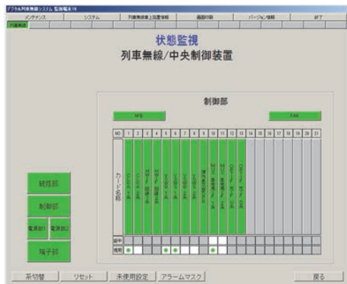
Fig. 9 Example screen of operation on supervisory (maintenance) terminal
