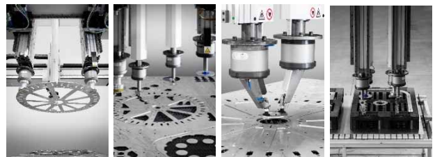
Fig. 7 An automatic sorting system picking up products
