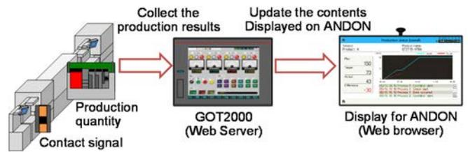
Fig. 2 Easy installation of ANDON system
