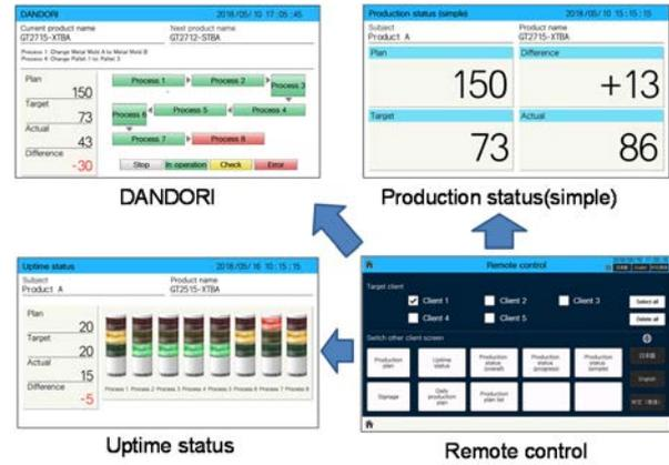
Fig. 6 Switching ANDON screens with remote control screen
