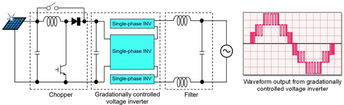
Fig. 2 Gradationally controlled voltage inverter
