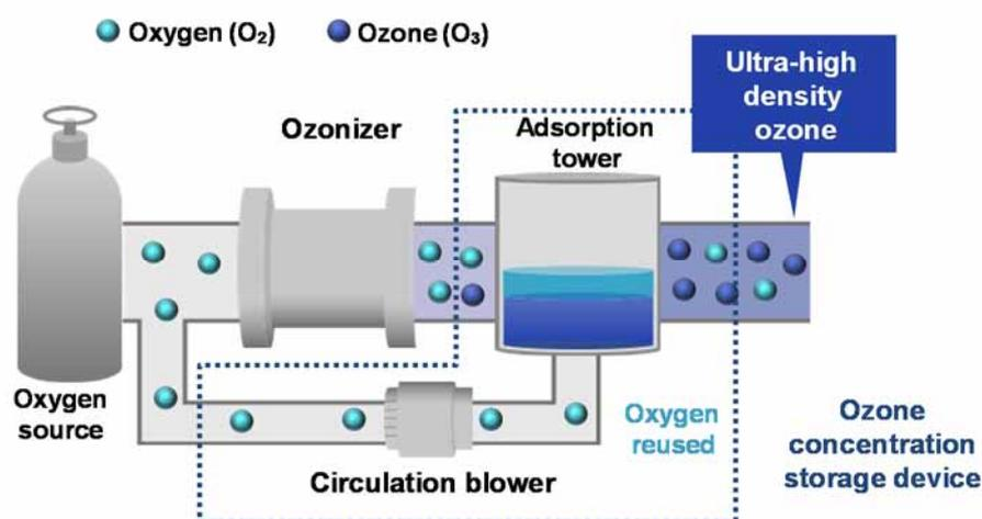
Fig. 1 Composition of ultra-high density ozone generation system
