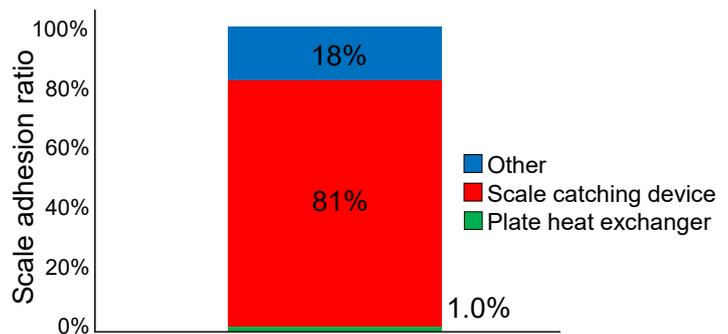
Fig. 3 Rate of scale deposition in the scale catching device demonstration test
