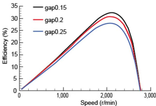
Fig. 2 Speed-efficiency characteristics
