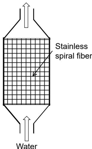
Fig. 2 Schematic of the scale catching device
