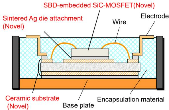
Fig. 2 Schematic cross section of the novel power module
