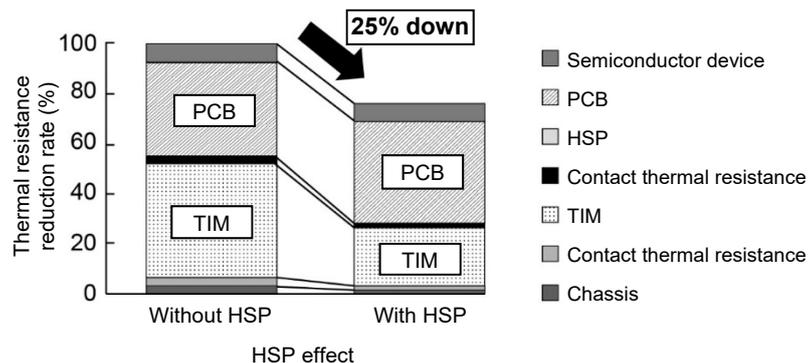
Fig. 4 Packaging structure using HSP and its effect
