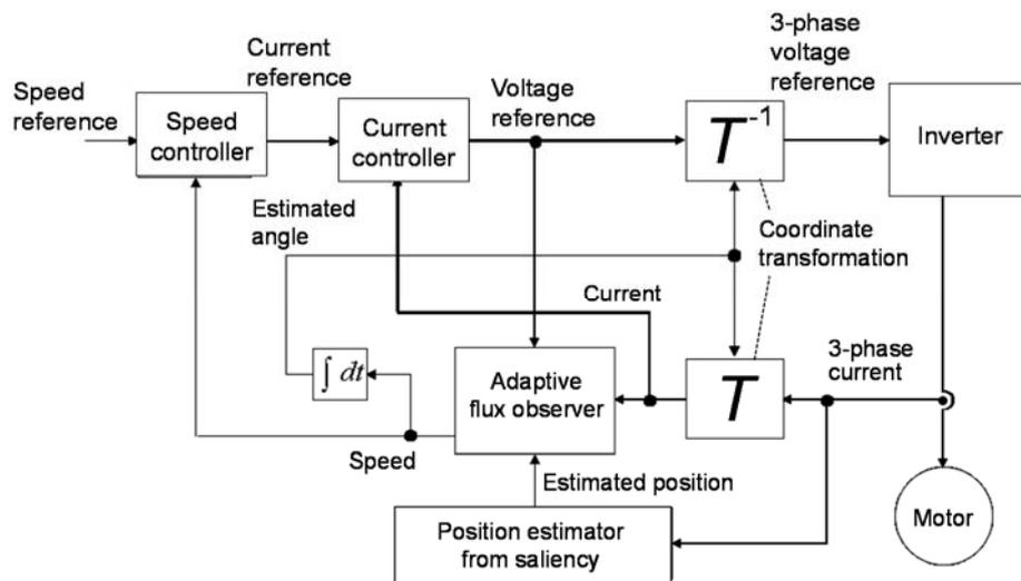
Fig. 1 Configuration of sensor-less servo control system
