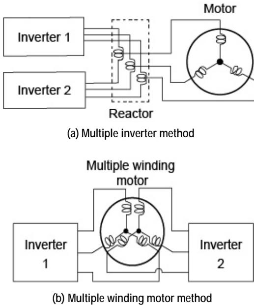
Fig. 3 Motor drive system controlled by multiple inverters
