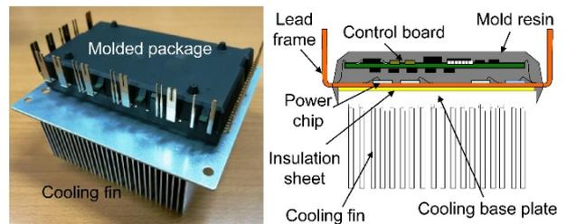
Fig. 4 High integration inverter
