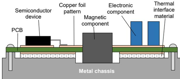
Fig. 2 Packaging structure using the TC-PAB technology
