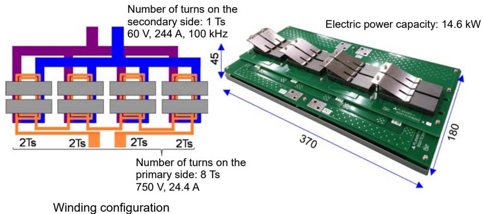
Fig. 6 Planar transformer
