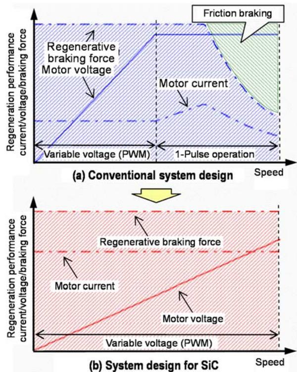
Fig. 5 Comparison of regenerative braking performance setting
