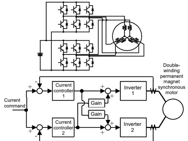
Fig. 5 Driving control of double-winding permanent magnet synchronous motor
