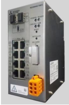
Fig. 2 Exterior view of the intelligent hub
