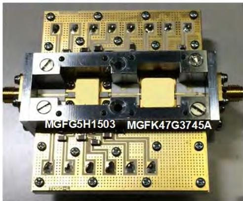
Fig. 7 2-stage Amplifier of MGFG5H1503 and MGFK47G3745A
