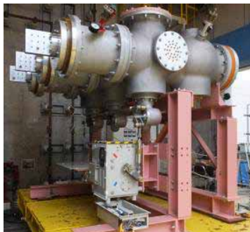
Fig. 9 Prototype 420 kV GIS under short circuit making test
