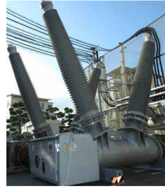
Fig. 10 Prototype 420 kV GCB under interruption test
