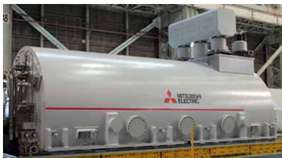
Fig. 1 870 MVA turbine generator used for verification test
