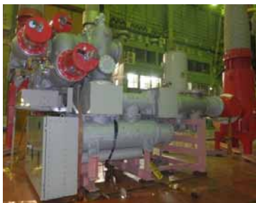
Fig. 8 Prototype 420 kV GIS under dielectric test
