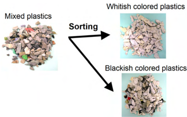
Fig. 7 Plastic flakes after color sorting process
