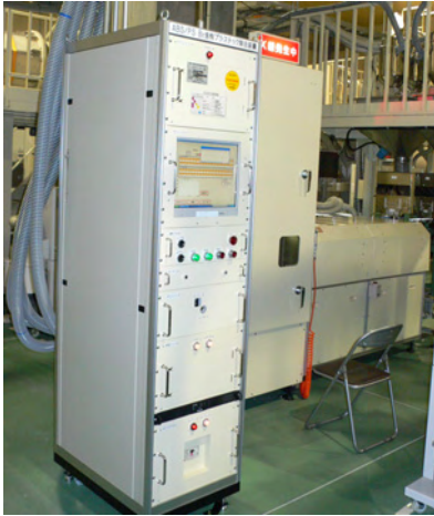
Fig. 4 Large-scale eliminating equipment for plastic flakes containing bromine
