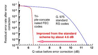
Fig. 7 Performance of triple-concatenated FEC codes
