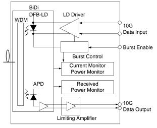
Fig. 6 Configuration of ONU optical transceiver
