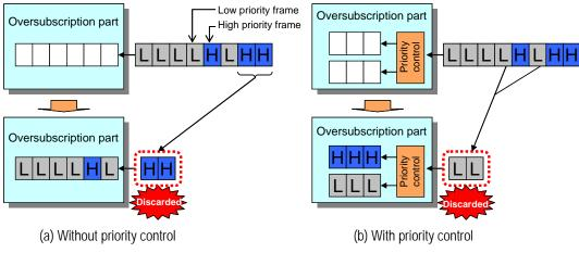
Fig. 6 Effect of priority control at the oversubscription part of the PON line card
