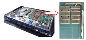
Fig. 1 Heat pipe mounted on the transponder
