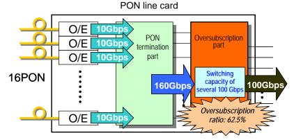
Fig. 5 Retaining and improving the oversubscription ratio for multiple ports
