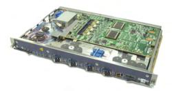
Fig. 6 External appearance of 40 Gbps muxponder for metro network applications
