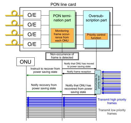
Fig. 7 Power saving by coordination between PON termination part and oversubscription part
