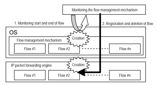
Fig. 6 Concept of fast-path forwarding control
