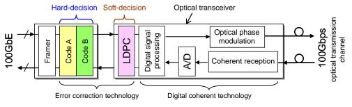
Fig. 8 Functional block diagram of 100 Gbps transponder
