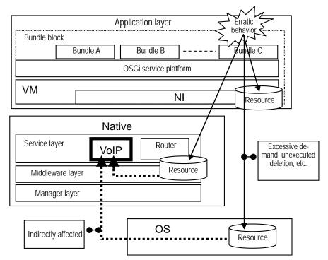
Fig. 5 Architecture of bundle block and threat to VoIP
