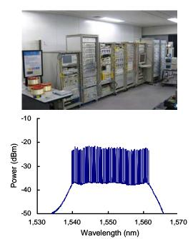
Fig. 3 Ultra long-haul transmission evaluation equipment (upper) and wavelength multiplexed spectrum after transmission over 9,000 km (lower)
