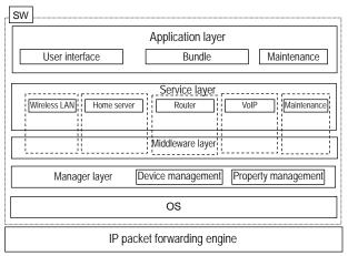
Fig. 2 Hardware architecture of HGW
