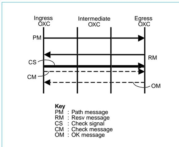
Fig. 5 Message sequence for optical path-continuity test
