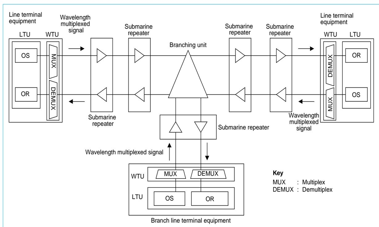
Fig. 1 Line terminal equipment
