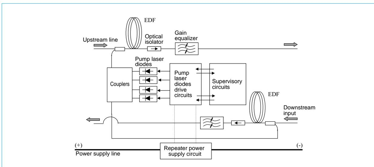
Fig. 3 Configuration of optical submarine repeater
