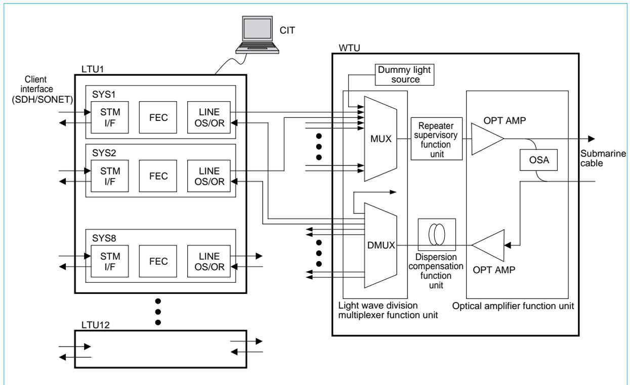
Fig. 6 System configuration of submarine line-terminal equipment
