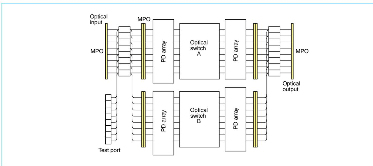
Fig. 2 Optical switching-plane architecture
