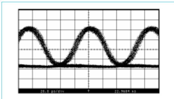
Fig. 7 Optical transmitted waveform.
