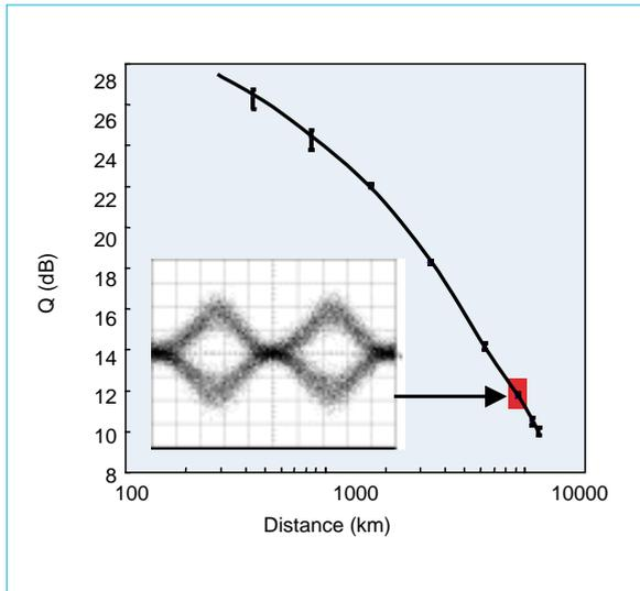
Fig. 1 Transmission performance of 10Gbps RZ-DPSK
