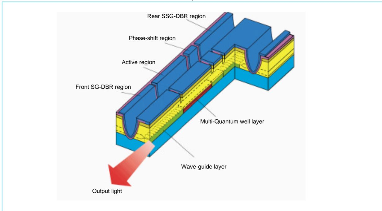
Fig. 1 Schematic of the SG-SSG-DBR laser
