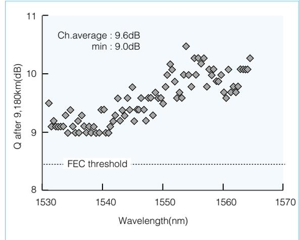
Fig. 5 Measured Q of 85 x 20Gbps signals after 9180km transmission
