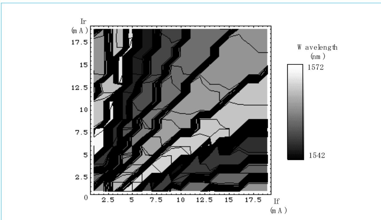
Fig. 2 Contour map of wavelength for DBR currents  $I_f$  and  $I_r$
