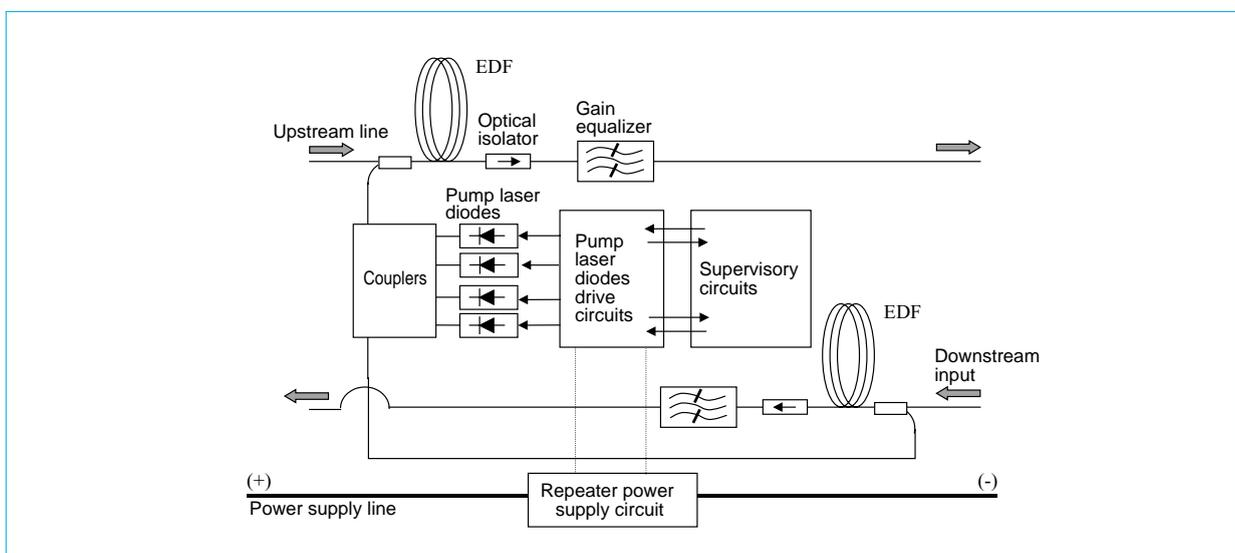
Fig. 3 Configuration of optical submarine repeater
