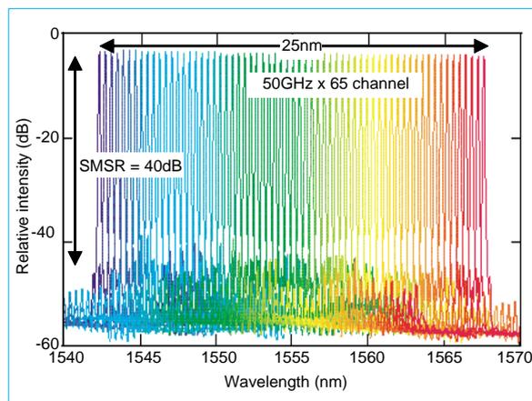
Fig. 3 Stabilized lasing wavelengths of the SG-SSG DBR laser
