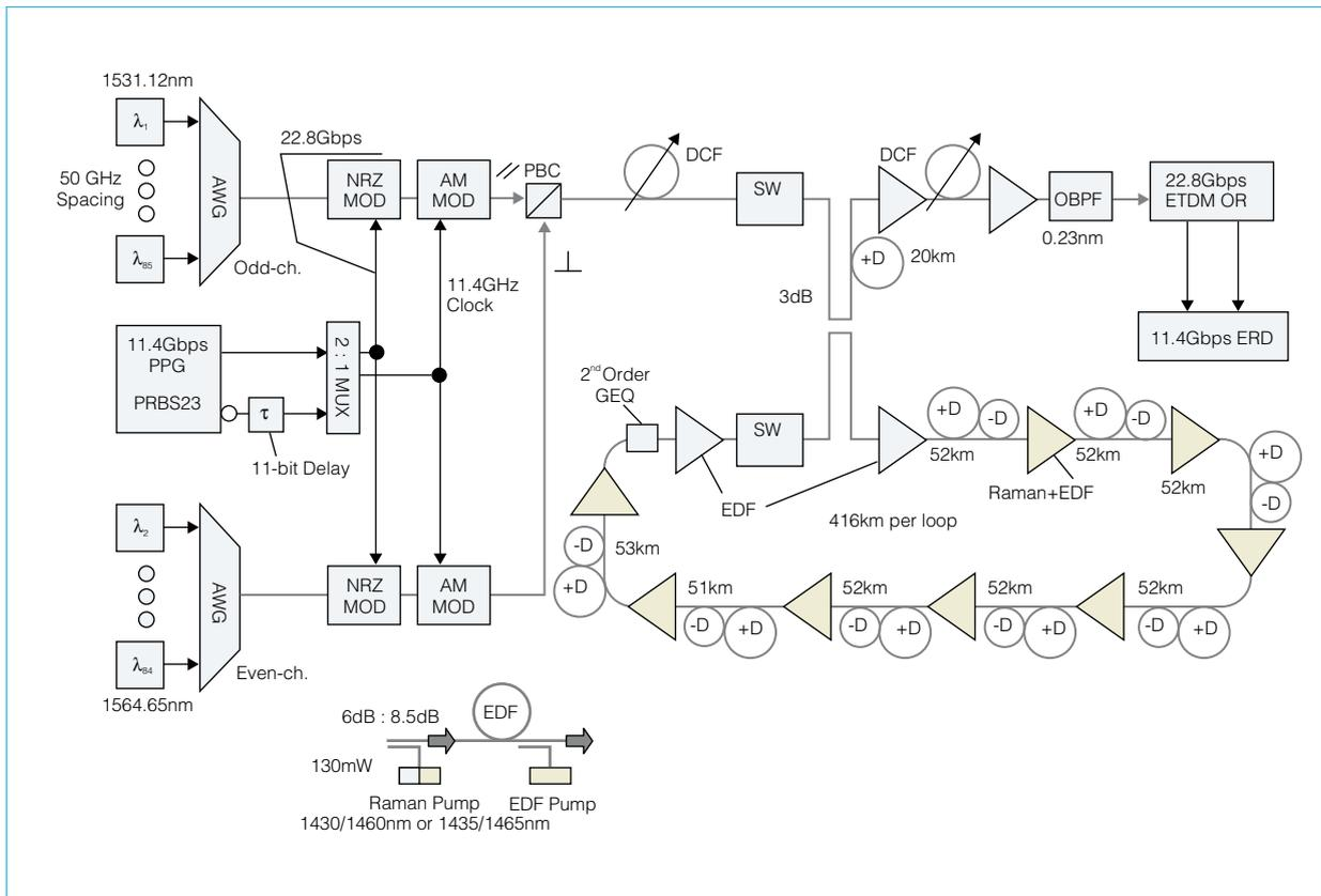
Fig. 4 Setup for 20Gbps x 85channels transmission experiment
