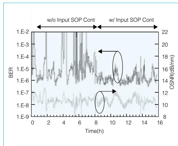
Fig. 3 Test result of PMD mitigation
