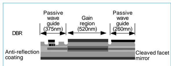
Fig. 4 Schematic of the mode-locked semiconductor laser structure
