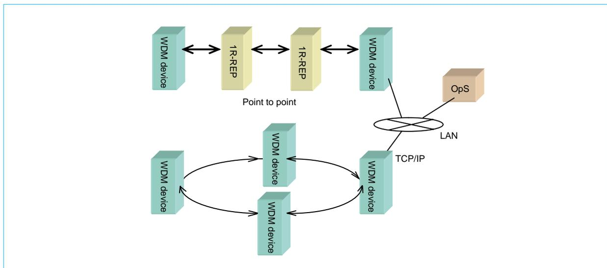
Fig. 2 WDM transmission equipment network topologies
