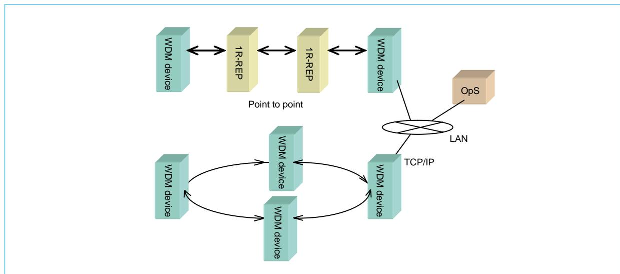
Fig. 2 WDM transmission equipment network topologies
