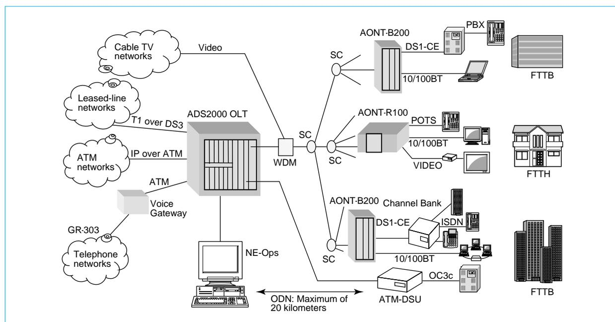
Fig. 1 The network configuration using an ATM passive optical network system
