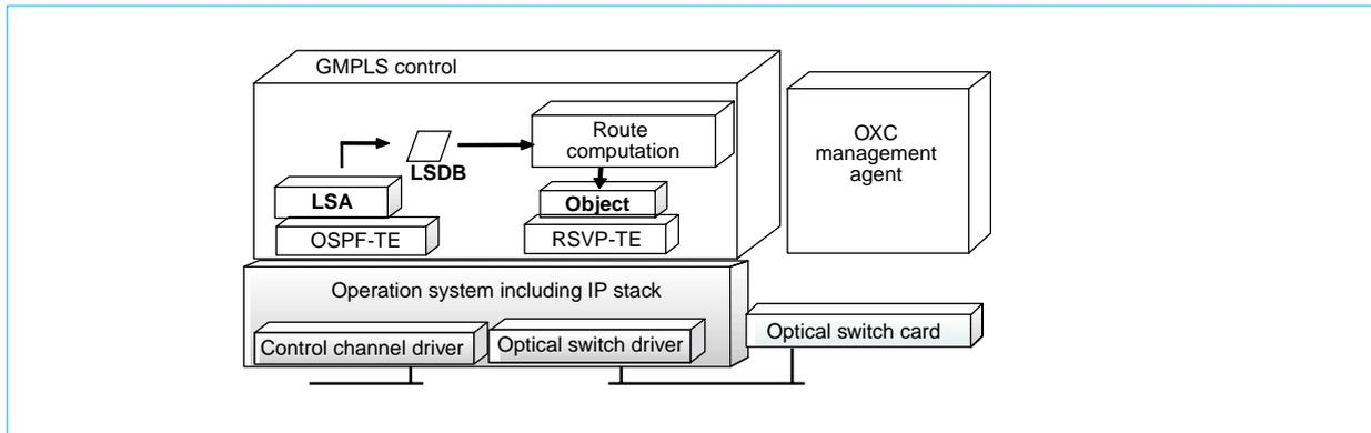
Fig. 3 OXC software architecture
