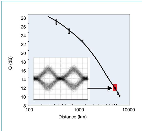
Fig. 1 Transmission performance of 10Gbps RZ-DPSK
