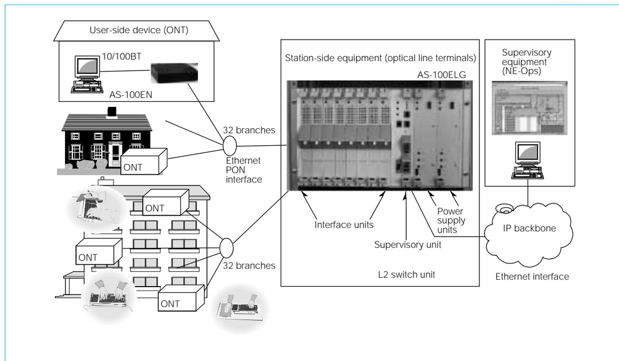
Fig. 4 The network configuration using an Ethernet passive optical network system
