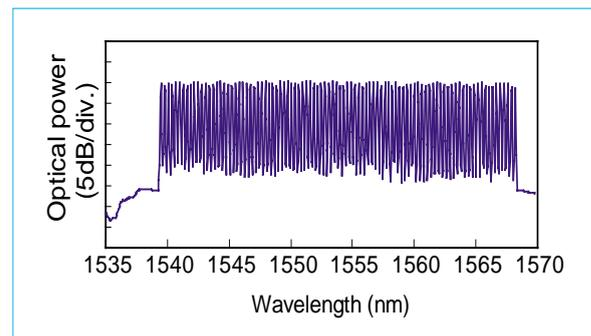
Fig. 4 Optical output spectrum of optical submarine repeater.
