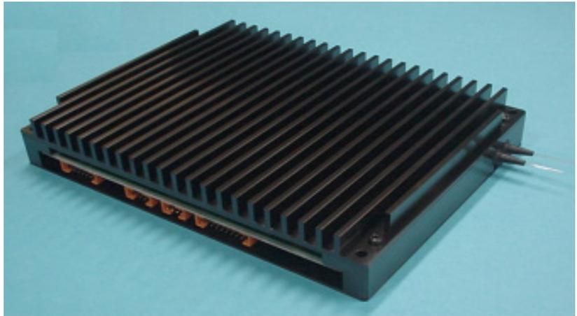
*Fig. 1 Tunable dispersion compensator*
