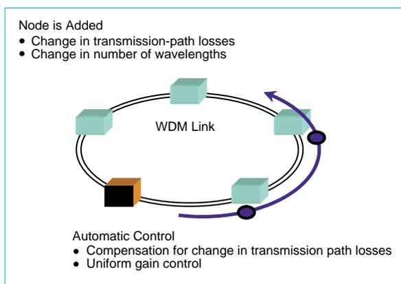
Fig. 4 *Transmission path-loss adjustments when a node is added*
