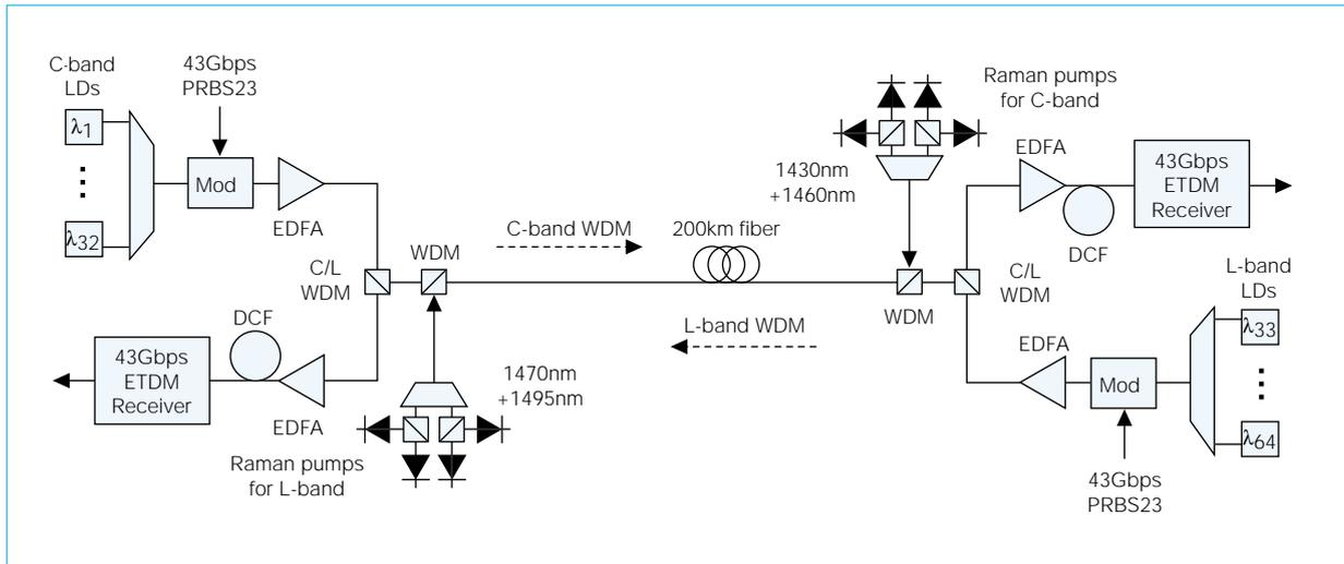
Fig. 6 Setup for 43Gps x 32 channels over 200km bidirectional
