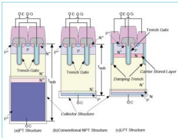
Fig. 1 Schematic cross section of various trench IGBTs.
