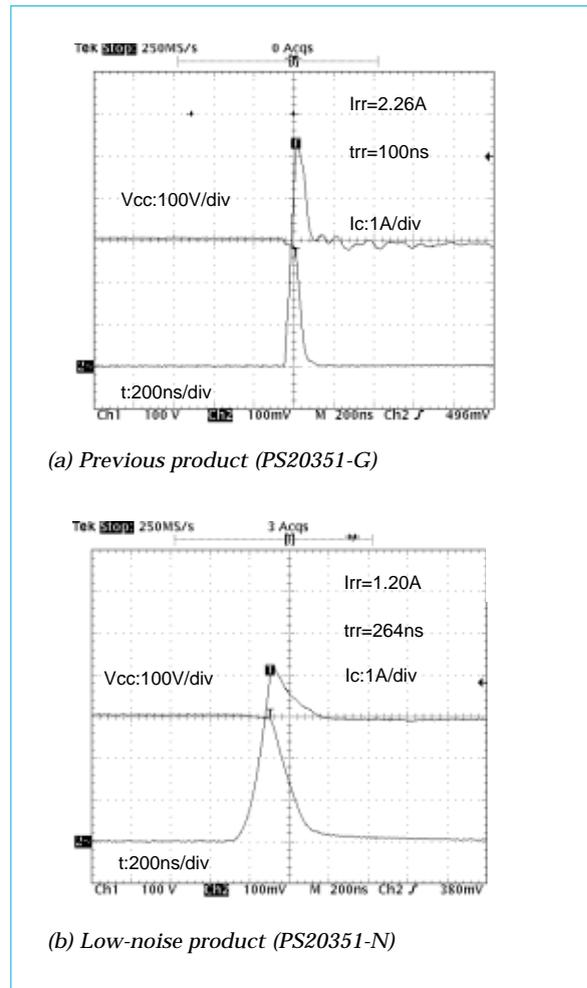
Fig. 4 Turn-on waveforms
