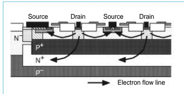
Fig. 3 Cross sectional view of DMOS(full isolation type)
