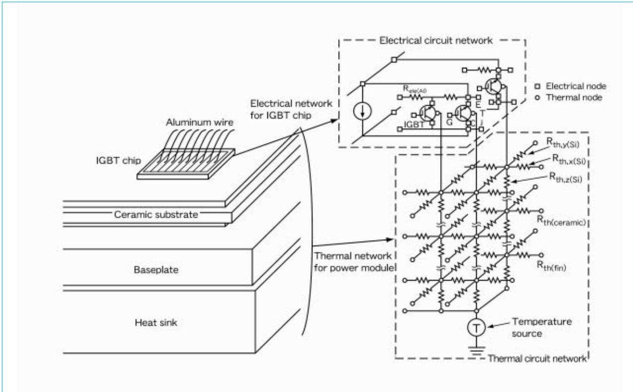
Fig. 6 Electrothermal network of an IGBT chip.
