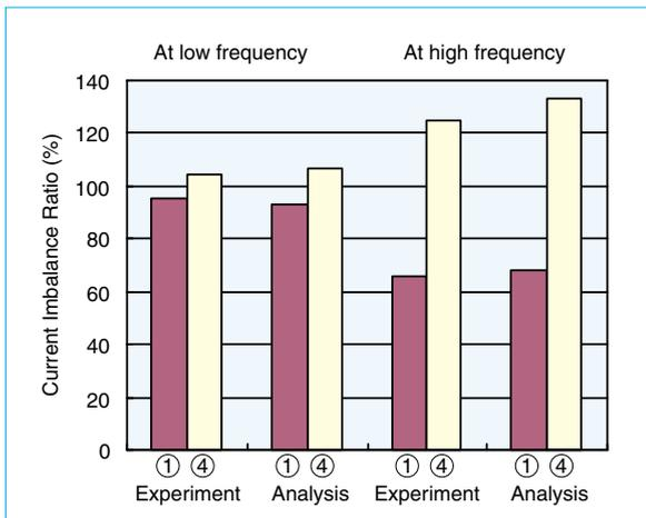
Fig. 3 Comparison of experimental and analytical results for chip current imbalance
