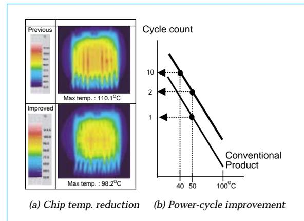
Fig. 5 Chip temp. reduction and power-cycle improvement
