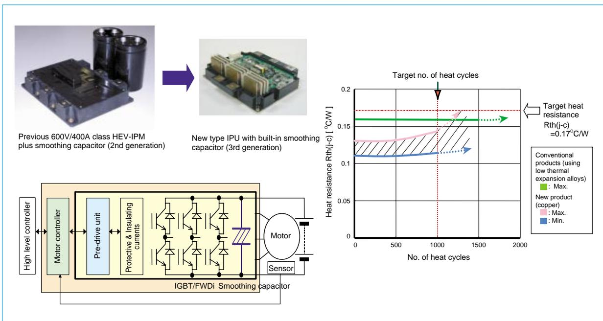
Fig. 7 Conventional HEV-IPM and IPU (prototype) at -40~125°C on a 15 x 15mm IGBT chip
