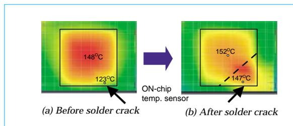
Fig. 4 Chip-temperature distributions.
