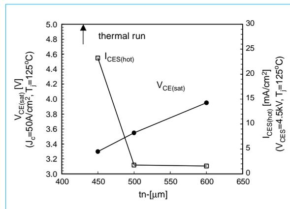
Fig. 2 Dependence of  $V_{CE(sat)}$  and  $I_{CES(hot)}$  on  $t_n$  in the 4.5kV-IGBT chip
