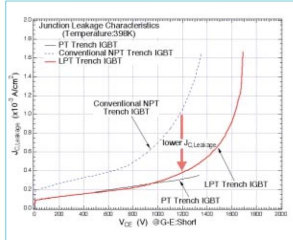
Fig. 4 Measured junction leakage characteristics of various trench IGBTs.
