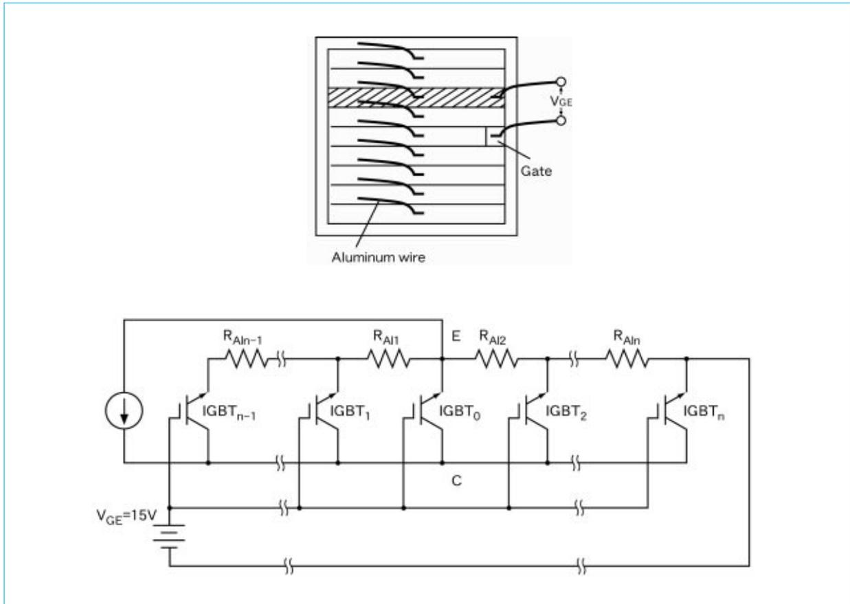
Fig. 4 Emitter surface of IGBT chip and electrical circuit model separating the IGBT chip into small IGBT segments
