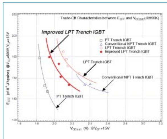
Fig. 7 Trade-off characteristics between on-state voltage ( $V_{CE(sat)}$ ) and turn-off loss ( $E_{OFF}$ ) for various trench IGBTs.
