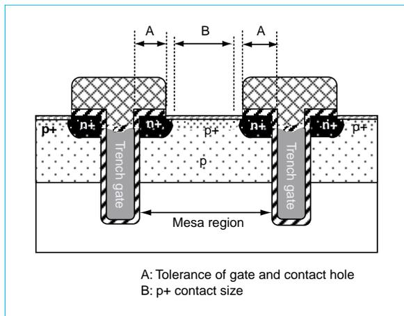
Fig. 2 The cross sectional view of the unit cell
