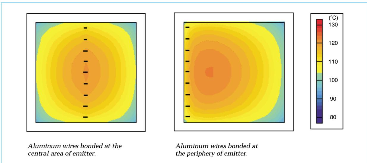
Fig. 7 Results of electrothermal simulation of the temperature distribution in an IGBT chip
