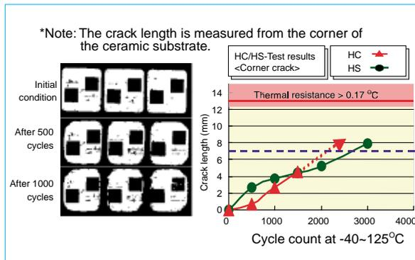
Fig. 3 Heat-cycle and heat-shock test results.
