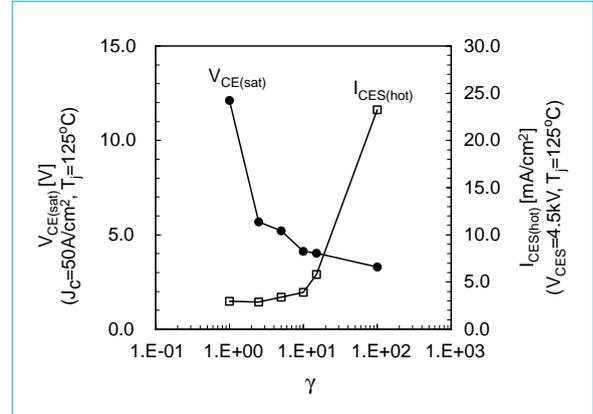
Fig. 4 Dependence of  $V_{CE(sat)}$  and  $I_{CES(hot)}$  on  $\gamma$  in the 4.5kV-IGBT chip
