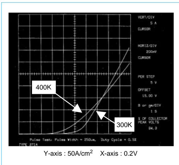
Fig. 6 IGBT ON-voltage characteristics
