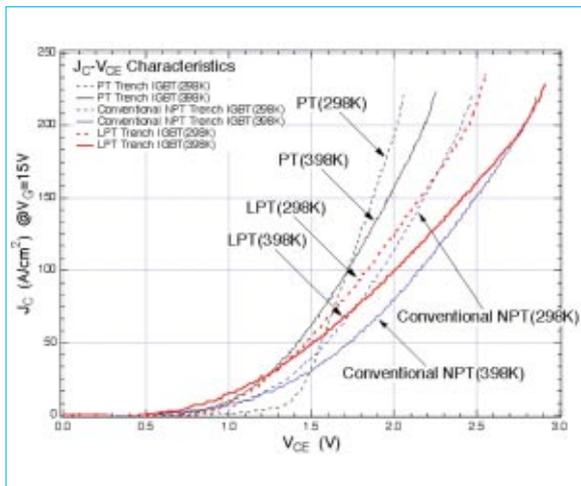
Fig. 3 Measured I-V characteristics of various trench IGBTs.
