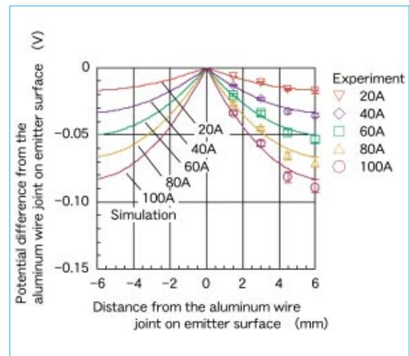
Fig. 5 Simulation results and measurements of potential distribution on the emitter surface.
