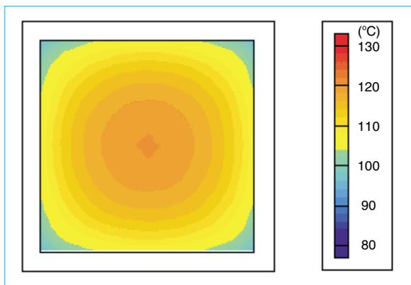
Fig. 9 Results of an electrothermal simulation of the temperature distribution of an IGBT chip, assuming uniform power dissipation
