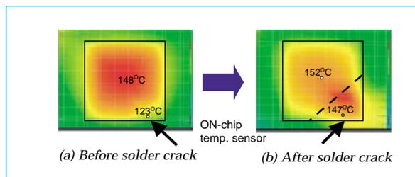
Fig. 4 Chip-temperature distributions.
