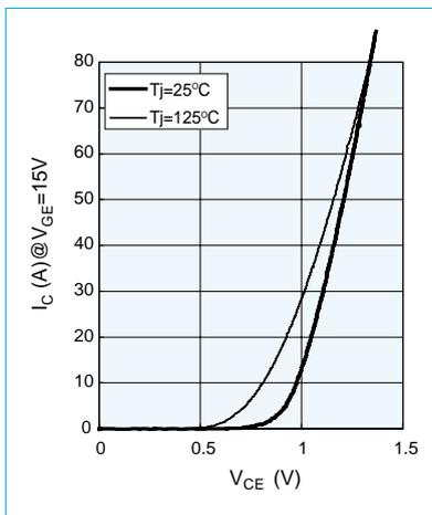
Fig. 3 I-V characteristics of CSTBT.
