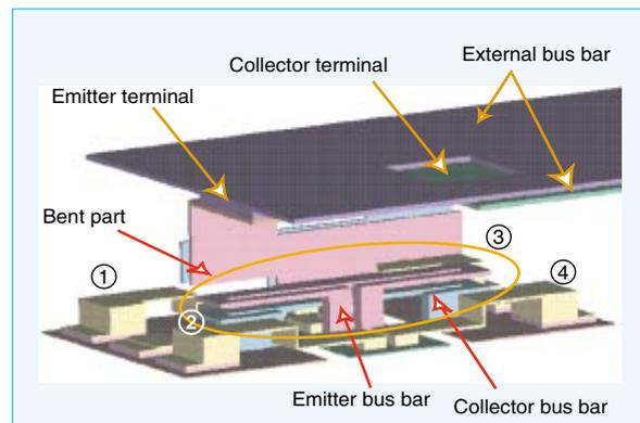
Fig. 1 Three-dimensional electromagnetic analysis model for power modules
