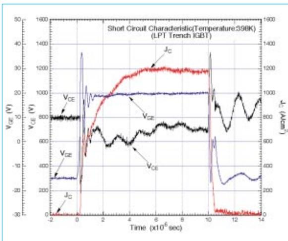
Fig. 6 Short circuit waveforms of 1200V LPT trench IGBT (@ $V_{CC}=800V$ ,  $R_C=2\Omega$ , 398K).
