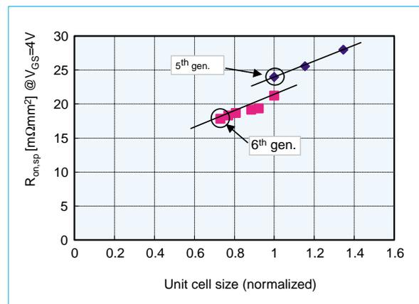
Fig. 1 The relationships between the normalized cell size and  $R_{\text{on,sp}}$
