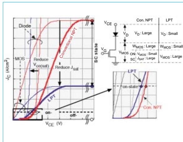
Fig. 2 Concept of wide cell pitch CSTBTs.
