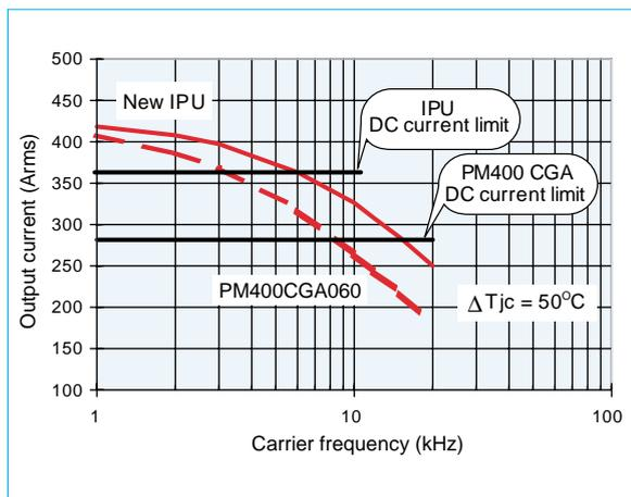
Fig. 8 IPU simulated output current capability
