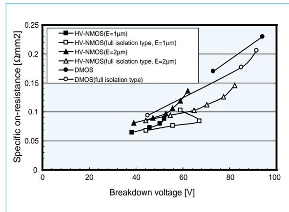
Fig. 5 Trade-off relation between specific on-resistance and breakdown voltage
