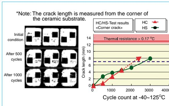
Fig. 3 Heat-cycle and heat-shock test results.
