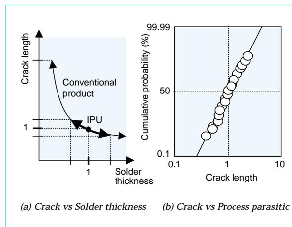
Fig. 2 Effect of solder thickness on the crack length
