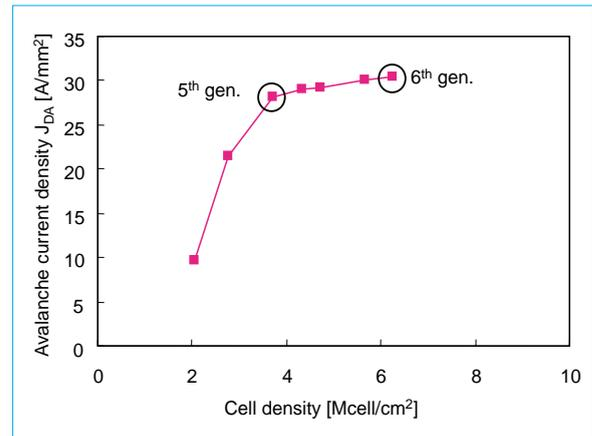
Fig. 3 Dependence of the avalanche current density on the cell density with the same p+ contact size.
