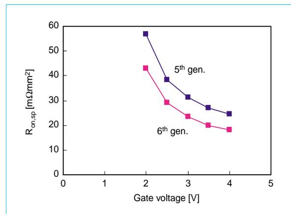
Fig. 4 Dependence of  $R_{on,sp}$  on the gate voltage.
