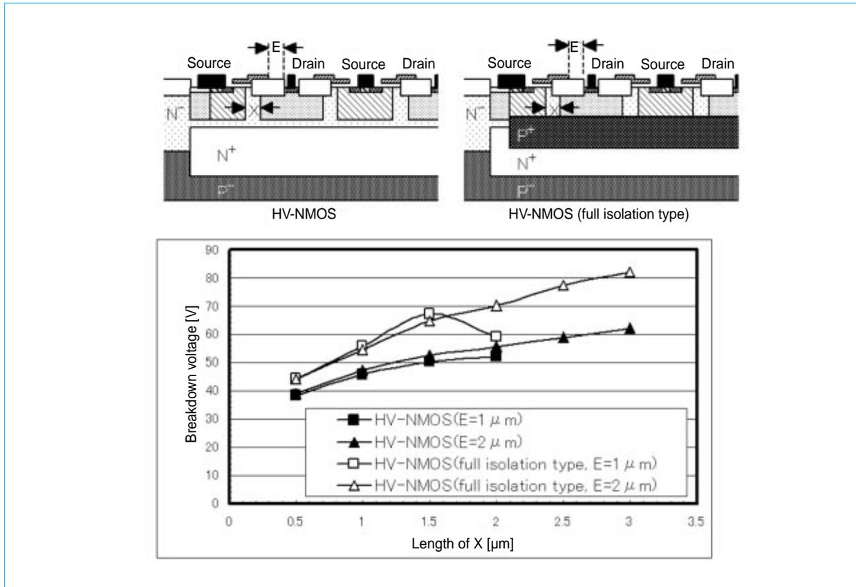
Fig. 4 Relation between the length X and the breakdown voltage
