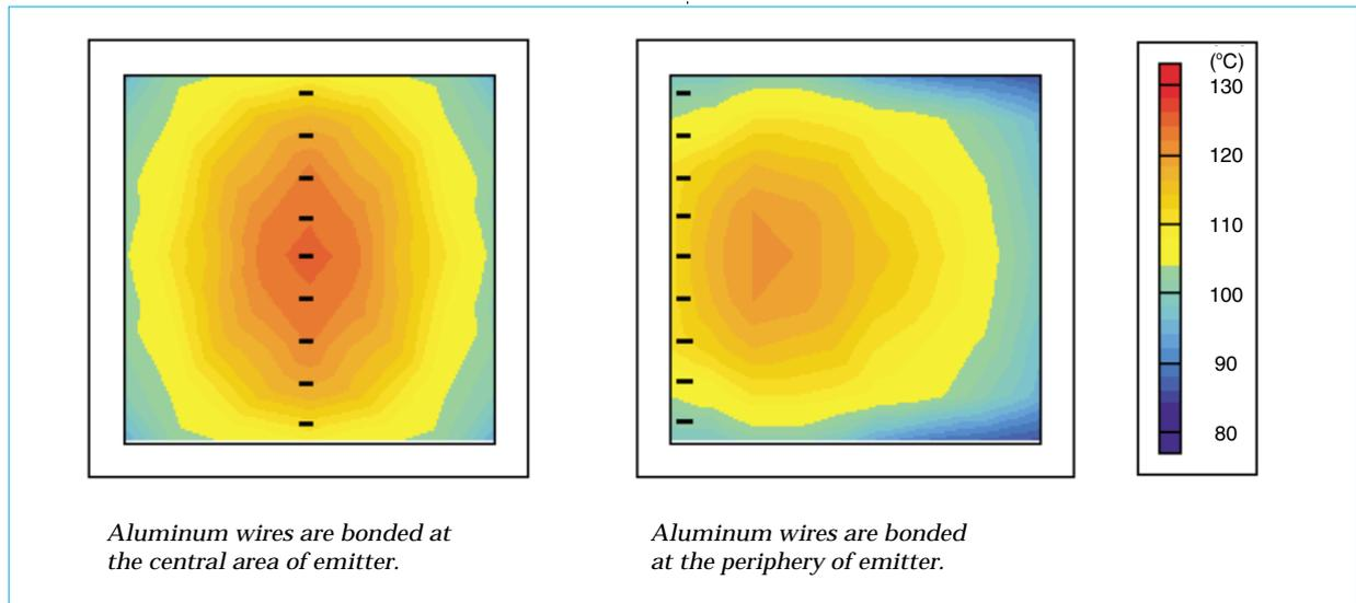
Fig. 8 The comparison of measured temperature distributions in IGBT chips with different wire bond positions
