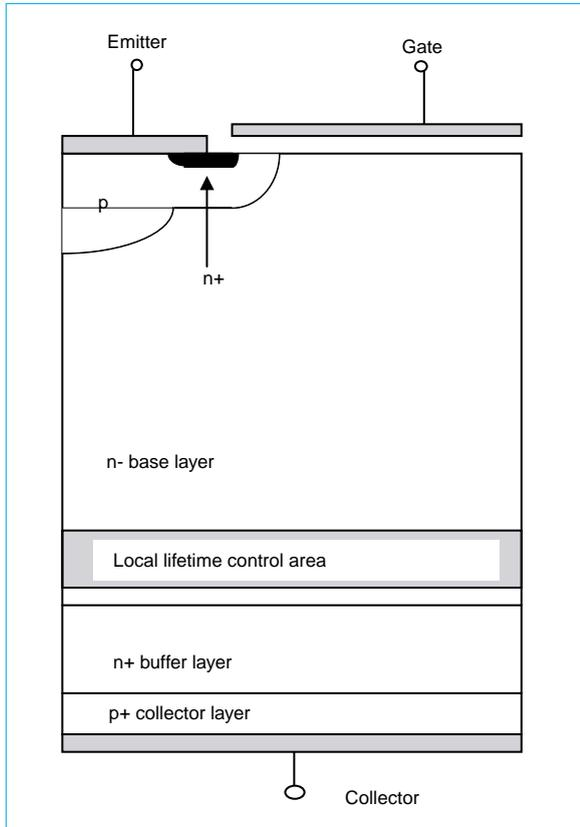
Fig. 3 Cross-section of the high-voltage IGBT chip
