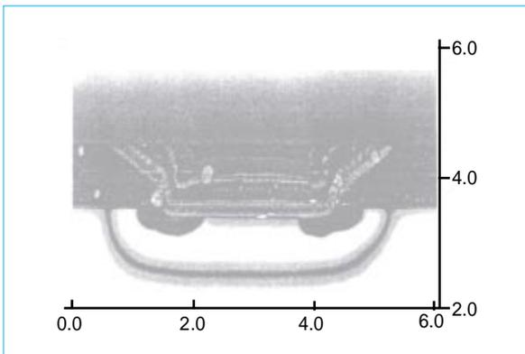
Fig. 2 SCM micrograph of DMOS cell (unit:  $\mu\text{m}$ )
