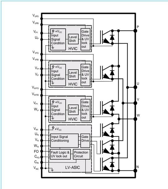
Fig. 3 Internal block diagram of the smaller transfer-mold DIP-IPM
