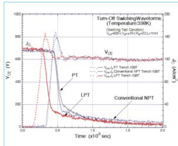
Fig. 5 Turn-off switching waveforms of various trench IGBTs under inductive load condition (@ $V_{CC}=600V$ ,  $V_{CE}\pm 15V$ ,  $R_G=2\Omega$ , 398K).
