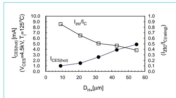
Fig. 5 Dependence of  $I_{CES}$  and  $I_{ztc}/I_C$  on  $D_{H^+}$  in the 4.5kV-IGBT chip
