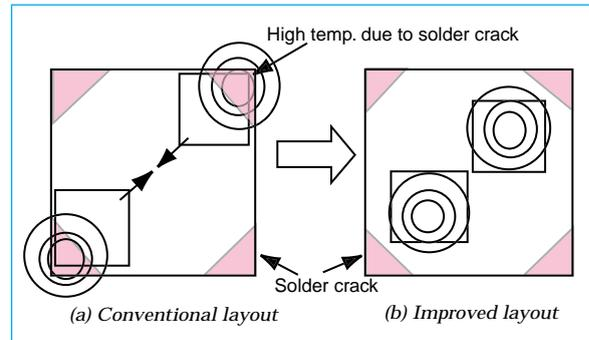
Fig. 1 Chip layout optimization
