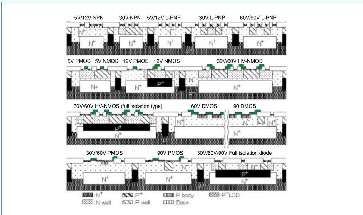
Fig. 1 Schematic views of main devices on BiC-DMOS
