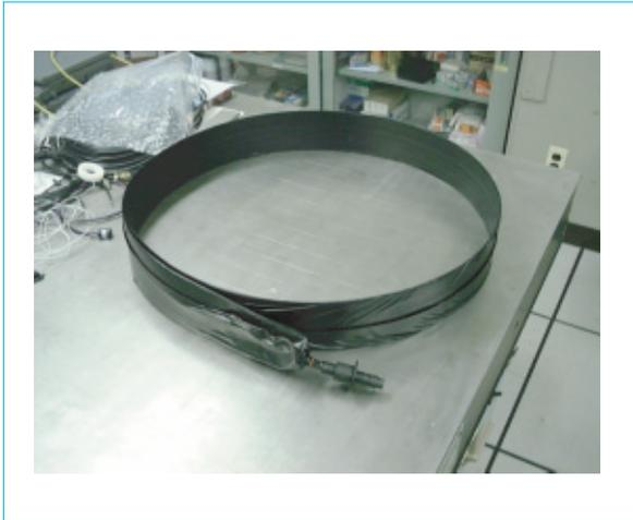
*Fig. 6 Scintillation fiber plate*
