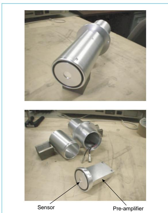
Fig. 2 Semiconductor beta-ray gas monitor
