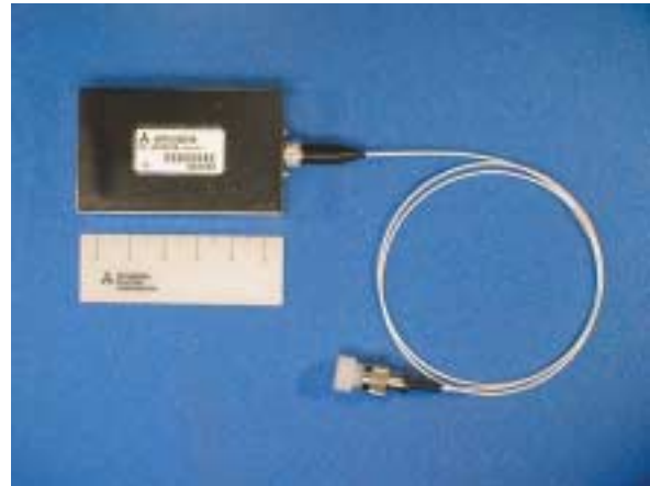
Fig. 1 ITU-T rec. G.957 L-16.3 optical transceiver
