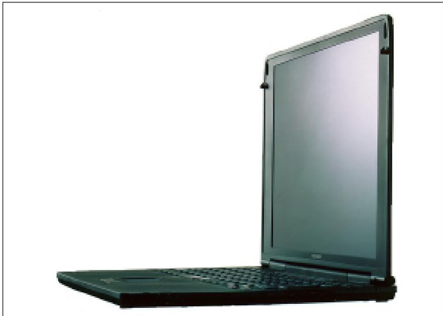
Fig. 1 This sleek notebook computer houses an LCD module just 6mm thick.
