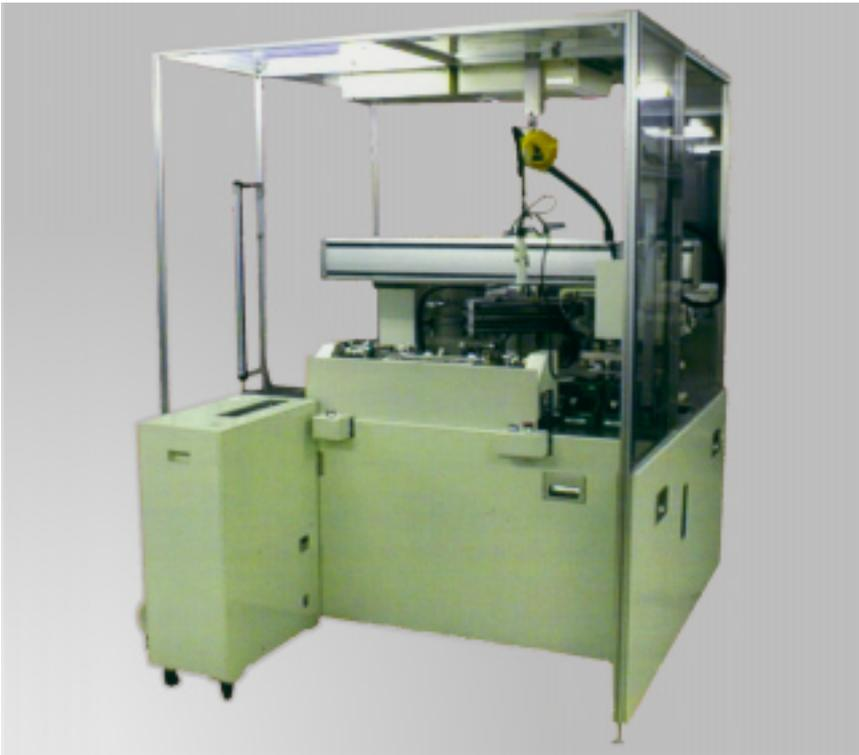
*Fig. 2 Assembly cell for thin LCD displays. The previous thickness of 20mm was reduced to 6.2mm.*
