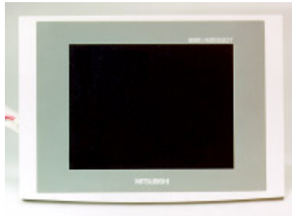
Fig. 1 The A850 graphic operation terminal developed by concurrent engineering.
